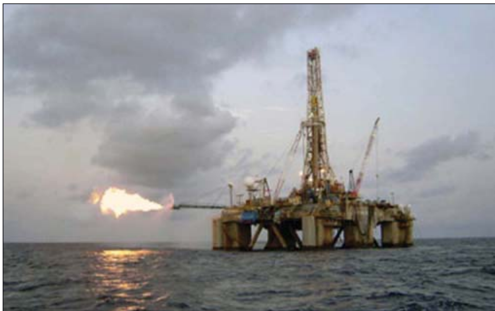
Toreador Resources Corp. was drilling off Turkey in the western Black Sea with the Atwood Southern Cross, a second-generation semisubmersible, shown flaring gas from the Akcakoca-3 well. The well tested about 34 MMcf/d from two of seven pay zones (Fig. 1, photo from Toreador Resources).
