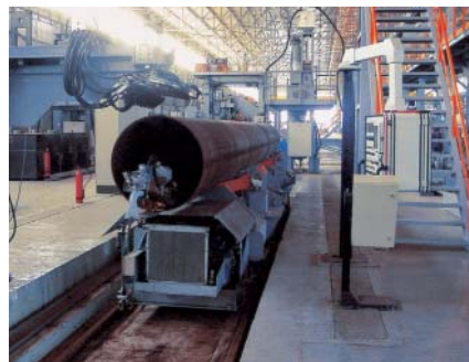
Ultrasonic testing machine, IPIC factory.
