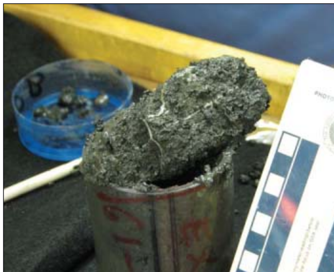
Gas hydrates are an ice-like combination of natural gas and water formed by high pressure and low temperatures. The expedition collected an “unprecedented” number of gas hydrate cores. Photo from USGS.
