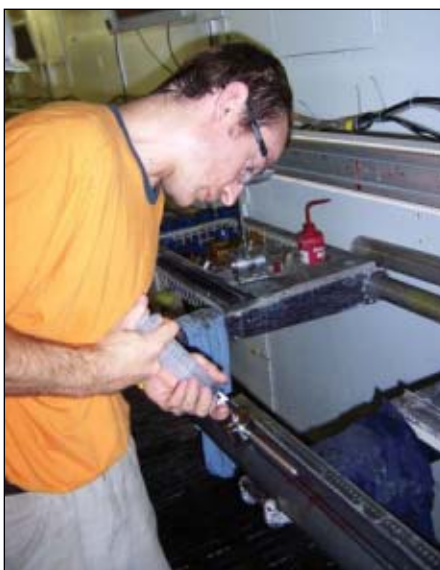
A technician measures the temperature of a core. The expedition recovered 494 cores with 2,850 m of sediment. Photo from USGS.
